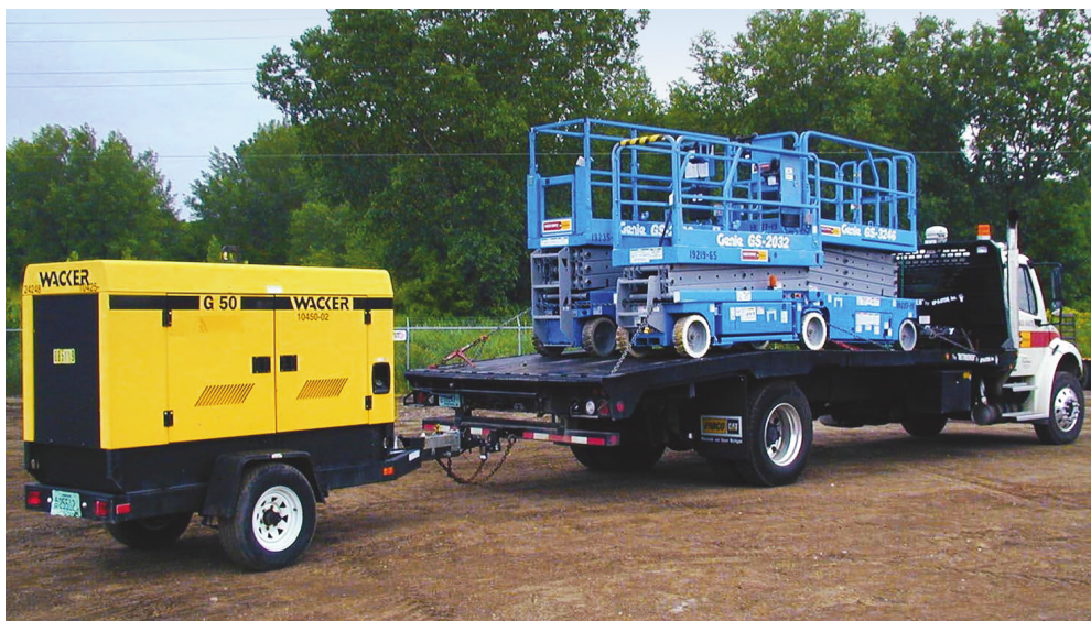
The Retriever low-profile truck bed features low deck height, light weight, and eliminates the need for a heavy, complex hydraulic system.
